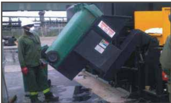
emptying general waste into compactor
