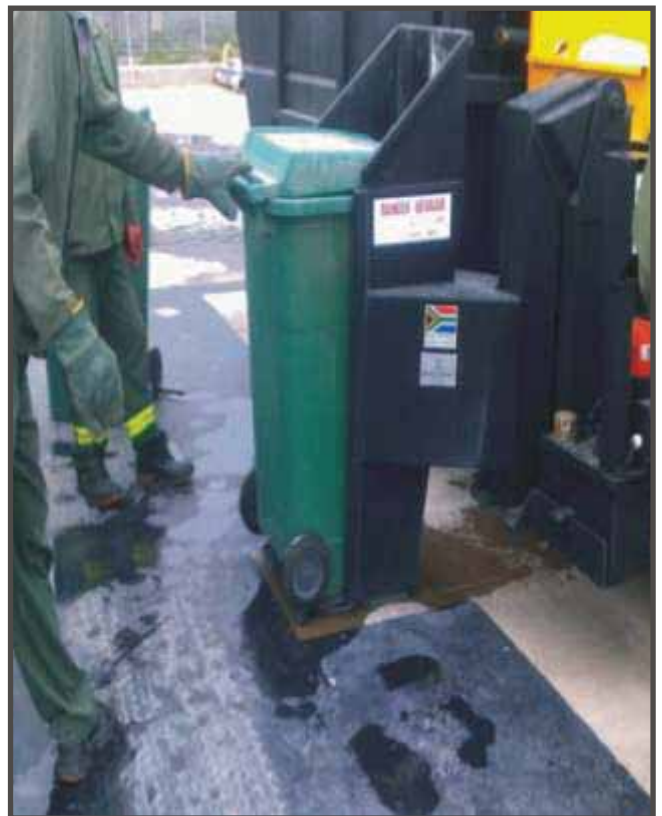
hooking up wheelie bin to compactor
